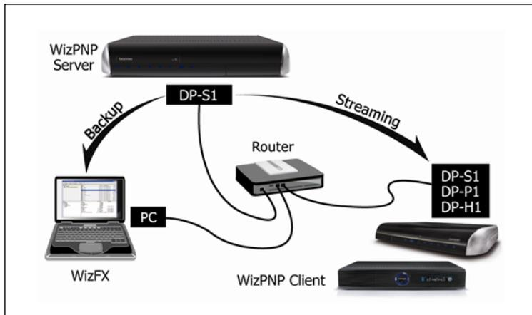
You can set the DP-S1 to be a WizPNP client, a WizPNP server, or both client and server simultaneously.
