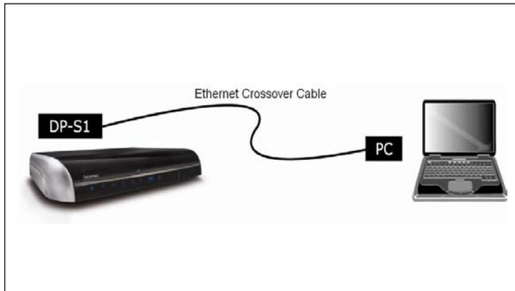
If your PC has the DHCP server feature and it is enabled, all the configurations for networking will be set automatically and the DP-S1 is ready to communicate with your PC. If your PC does not have the DHCP server feature, you must disable the DHCP feature and set IP (Internet Protocol) information manually for the DP-S1 and PC. For more information on manually configuring DHCP, please refer to Chapter 4 "Quick Setup".
