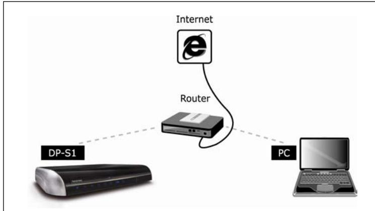
As shown in the picture, connect the DP-S1 to the router through your wireless network. If you purchase a wireless router with a DP-S1 and have no experience of connecting a wireless router with a PC, please refer the user's manual of the router and connect the DP-S1 to the router in the same manner as an additional PC. For more information on configuring WLAN please refer to Chapter 4 "Quick Setup"
