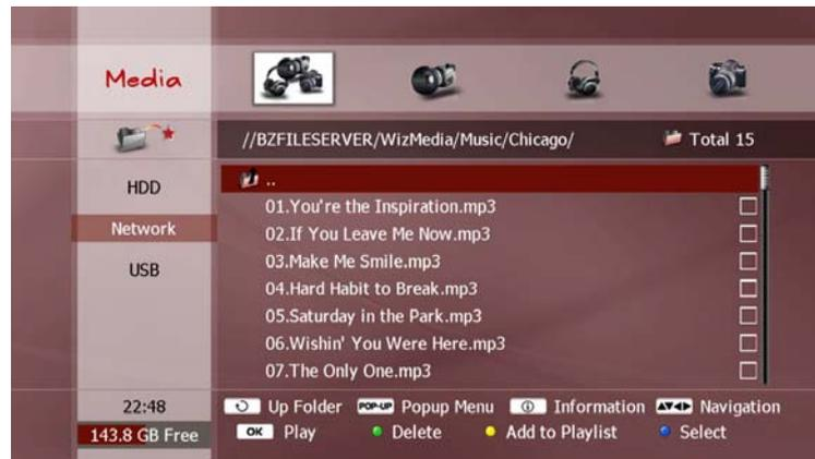
To choose a particular selection of files, select a desired file and press the **BLUE** button. A tick will appear in the box alongside the selected file. Repeat this procedure for the remainder of your selection.
