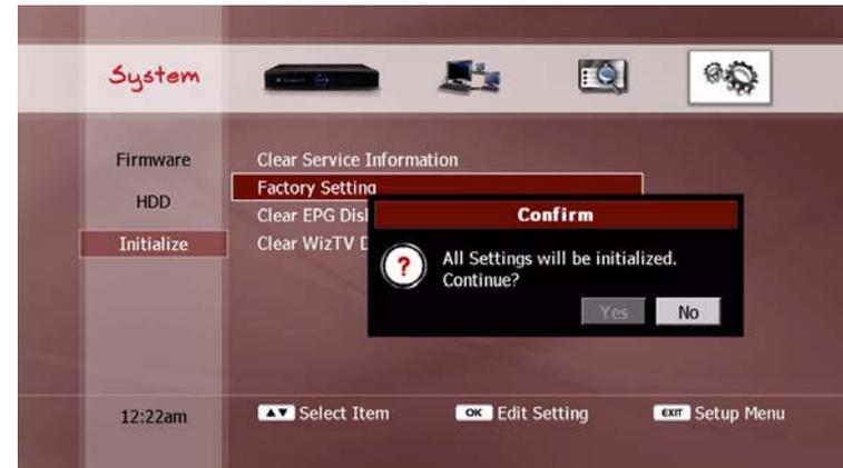
Select "Yes" and press the **OK** button to proceed. To cancel the factory setting function, select "No" and press the **OK** button, or press the **EXIT** button.
