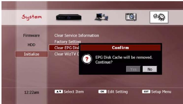
Select “Yes” and press the **OK** button to proceed. To cancel the clear IceGuide disk cache function, select “No” and press the **OK** button, or press the **EXIT** button.
