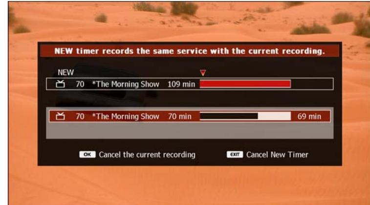
In order to allow the timer to begin, you must stop the current recording by pressing the **OK** button. If you don't wish to stop the current recording, press **EXIT** to cancel the pending timer.
