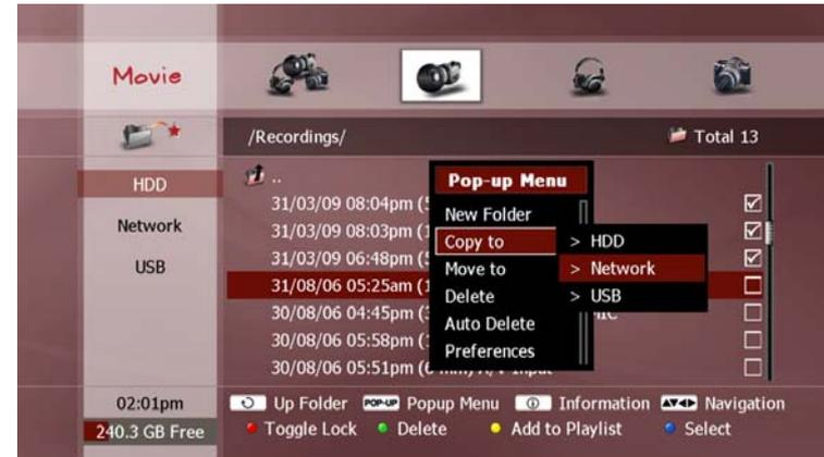
Use the **UP/DOWN** buttons to select the type of storage device for your desired destination and press the **OK** button. A pop-up browser window will appear.
