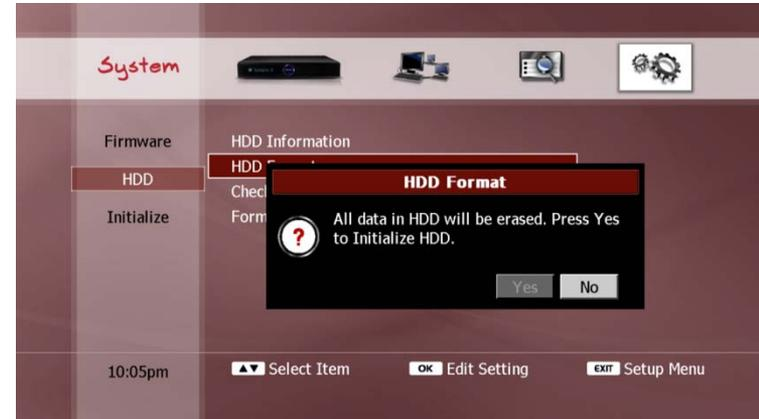
Select "Yes" and press the **OK** button to proceed. To cancel the HDD format function, select "No" and press the **OK** button, or press the **EXIT** button. If you select "Yes", the DP-Lite will restart and format the internal HDD automatically.
