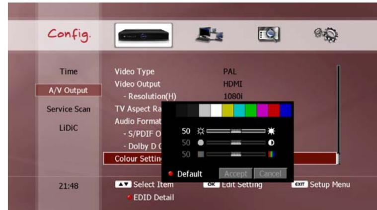
The three options are brightness, contrast and saturation. Use the **UP/DOWN** buttons to select each option, and adjust the setting with the **LEFT/RIGHT** buttons. You can restore all colour settings to the factory default values by pressing the **RED** button. To apply your chosen settings, use the **UP/DOWN** buttons to select “Accept” and press **OK**. To cancel the new settings, select “Cancel” and press **OK**, or press the **EXIT** button.
