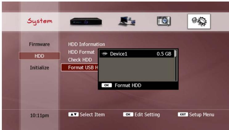
Use the **UP/DOWN** buttons to select the device you wish to format and press the **OK** button.
