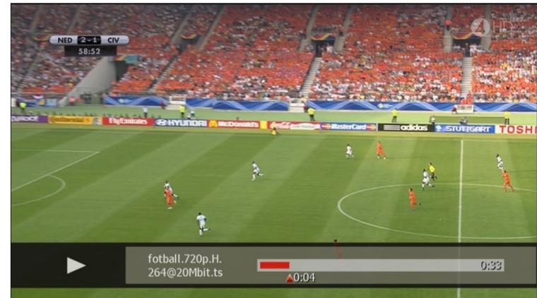
You can also display the progress bar at any time by pressing the **OK** button. To hide the progress bar, press the **OK** button again, or **EXIT**.
