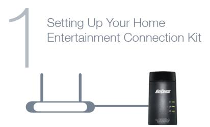
Connect one end of the supplied Ethernet cable into the LAN Ethernet port of your modem/router.
