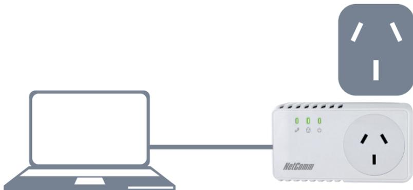
Connect one end of the other supplied Ethernet cable into the Ethernet port of any device you want to connect to the Internet (PC, set-top box, gaming console, PVR, blu-ray player etc).
