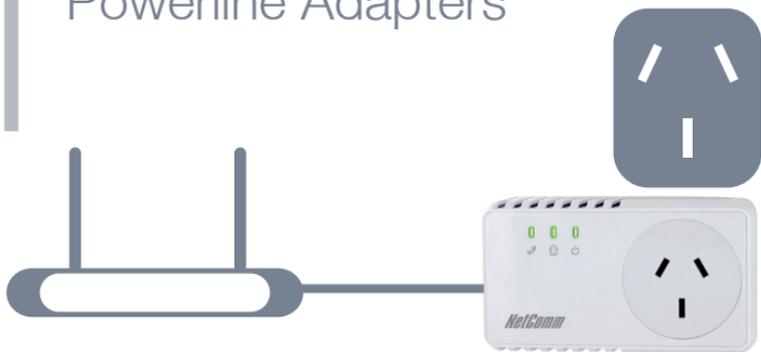
Using one of the supplied Ethernet cables connect one end into the LAN Ethernet port of your modem/router.
