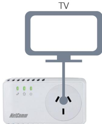
At this point, you can plug another electrical appliance into the Powerline Adapters AC pass-through if you wish to do so.
