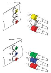
You need to obtain a Composite cable (RCA cable) to use the Composite connector. Plug one end of the cable into the VIDEO (yellow), AUDIO L (white) and AUDIO R (red) sockets on the digital receiver, and plug the other end into the matching socket on your video recorder or suchlike.
