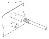
Whatever sort of connection you have between the digital receiver and the television, you need to connect the digital receiver to the antenna so that it can receive digital television broadcasts. Connect the antenna cable to the ANT IN connector. If you have another digital receiver, you may link it from the ANT OUT connector.
