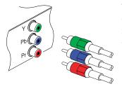
You need to obtain a component video cable (RCA cable) to use the component video connector. Plug one ends of the cable into the Y (green), Pb (blue) and Pr (red) sockets on the digital receiver, and plug the other ends into the matching sockets on your television.
