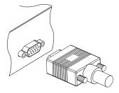
You need to obtain a RGB cable (15 pin D-sub cable) to use the RGB connector. Plug one end of the cable into the RGB socket on the digital receiver, and plug the other end into the matching socket on your television.
