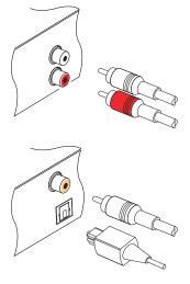
You need to obtain an audio cable (RCA cable) to connect the audio connectors. Plug one end of the cable into the AUDIO L (white) and AUDIO R (red) sockets on the digital receiver, and plug the other end into the matching sockets on your television or audio system.
