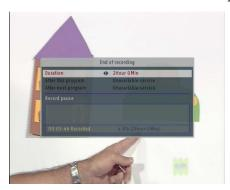
Once a recording is started, pressing the button displays a menu like the left figure, in which you can set the recording duration, or pause the recording. To specify an arbitrary recording duration, set the Duration option as you desire with the V— and V+ buttons and press the OK button; the recording will end at the specified time.
