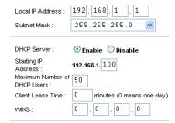
You can let the router automatically assign a dynamic IP address to the computers or devices connected to the network by enabling the DHCP server of the router. In this case, you can access the digital receiver with the IP address which is assigned to the digital receiver by the router.
