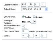
You can let the router automatically assign a dynamic IP address to the computers or devices connected to the network by enabling the DHCP server of the router. In this case, you can access the digital receiver with the IP address which is assigned to the digital receiver by the router.
