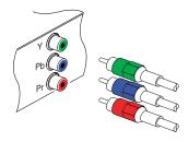
You need to obtain a Component video cable (RCA cable) to use the Component video output. Plug one ends of the cable into the Y (green), Pb (blue) and Pr (red) sockets on the digital receiver, and plug the other ends into the matching sockets on your television.
