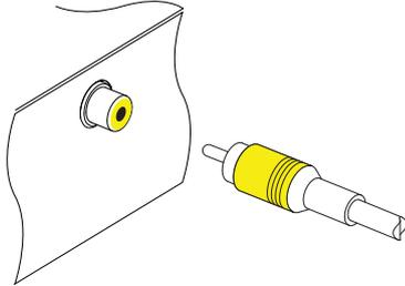
You need to obtain a Composite video cable (RCA cable) to use the Composite video output. Plug one end of the cable into the VIDEO (yellow) socket on the digital receiver, and plug the other end into the matching socket on your television.
