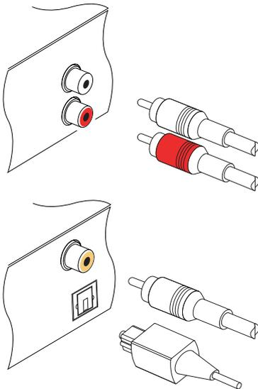
You need to obtain an audio cable (RCA cable) to link the audio connectors. Plug one ends of the cable into the AUDIO L (white) and AUDIO R (red) sockets on the digital receiver, and plug the other ends into the matching sockets on your television or audio-video receiver.
