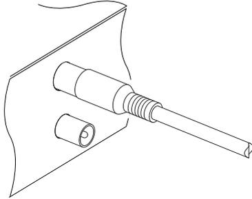
Whatever sort of connection you have between the digital receiver and the television, you need to connect the digital receiver to the antenna so that it can receive digital television broadcasts. Connect the antenna cable to the ANT IN connector. If you have another digital receiver, you may link it from the ANT OUT connector.
