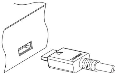
If you have a high definition television set, you should use an HDMI cable for best results. Plug one end of the cable into the HDMI socket on the digital receiver, and plug the other end into the matching socket on your television. In this case, you do not have to make audio connection because it can output stereo audio or digital audio as well.
