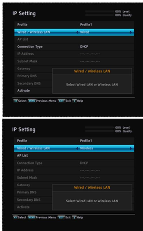
Head down to **Wired/Wireless LAN** and use the **Right** key button to change it to **Wireless**.
