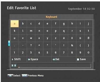
You can move the highlight key horizontally with the **( $\odot$ )** and **( $\ominus$ )** buttons and vertically with the **( $\odot$ )** and **( $\ominus$ )** buttons. Pressing the **(OK)** button on a key enters its letter in the input line. To type a space, select the **Space** key. To type lower case letters or numerals, select the **Shift** key.
