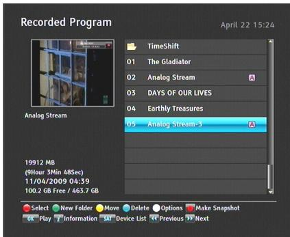
Select the Recording > Recorded Program menu or alternatively press the
