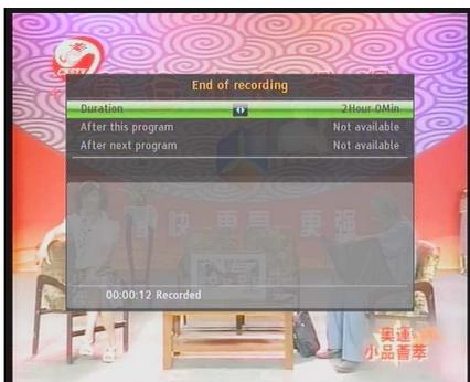
After a recording has started, pressing the
