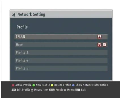
After you finish making network profiles, activate an available profile with the
