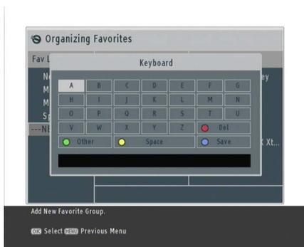
You can move the highlight key horizontally with the **[V-]** and **[V+]** buttons and vertically with the **[P+]** and **[P-]** buttons. Pressing the **[OK]** button on a key enters its letter in the input line. To type a space, select the **Space** key or press the **[Space]**. To type lower case letters or numerals, select the **Other** key or press the **[Other]**.
