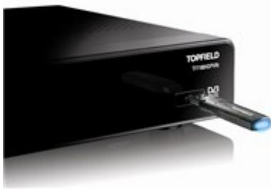
Remove flap and insert wireless USB dongle.
